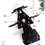
Disassemble the original plate holder, the rear light and arrows. Keep the original screws to reuse them later.
